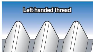
A thread which, when viewed axially, winds in a counter clockwise and receding direction. All left handed threads are designated LH
